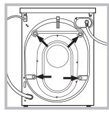
3. Remove the 4 protective screws and the rubber bush with the respective spacer, situated on the rear of the appliance (see also the installation leaflet). 4. Seal the gaps using the plastic plugs provided.
